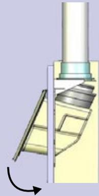
Align the four holes in the valve assembly with the holes in the frame. Secure with the four screws provided with the trim kit.
