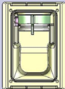
Install the door by lining up the door and valve hinge while pressing it gently into place.
