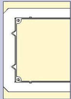
Push the two bottom pointed tabs into the sheet rock. The top pointed tab can be bent down as you pull the top of the frame into the hole.
