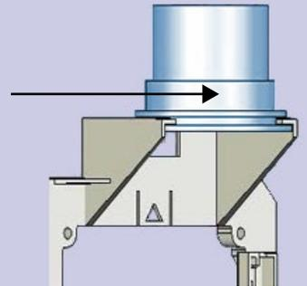
Install the pipe into the fitting. Glue the pipe into the fitting, ensuring that it seats all the way to the ridge of the pipe fitting.
