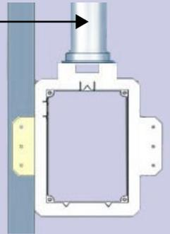
The pipe fitting is designed to slide in the frame to adjust for any variations in the thickness of the wall board. The maximum wall thickness that the valve can adjust to is 1,9 cm (3/4").
